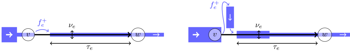
Figure 1: An edge with congestion modelled using the Vickrey point queue model. If the edge inflow rate f_e^+ is smaller than the edge capacity \nu_e , flow traverses the edge without experiencing any congestion (left). If the inflow rate is larger than the capacity, a queue forms at the tail of the edge (right).
